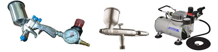
The kit contains an HVLP gun with regulator and ¼" quick-disconnect fittings to connect to shop or tank air supply. An airbrush and airbrush compressor with air fittings is included for painting smaller models or calibration samples. Each of the academic PSPs and TSPs are included in 12-oz aerosol spray cans for easy application and practice of the PSP technique. More advanced BinaryFIB® pressure sensitive paint and FIB Basecoat for research quality data is also included in the kit.
