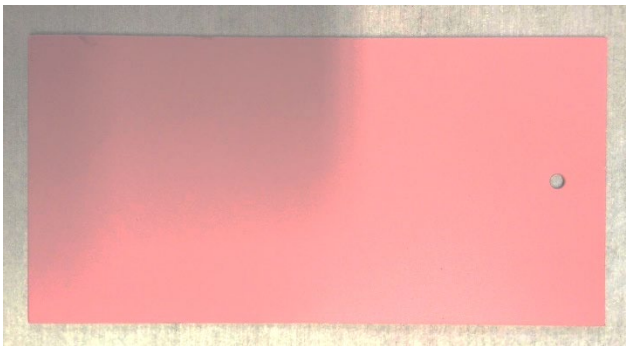
Aluminum Test Model Painted with PSP
