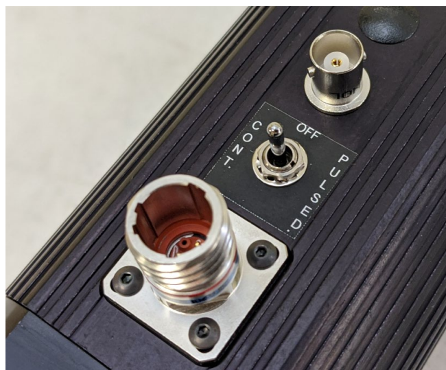
Trigger Switch on LM2X-DM LED Module
