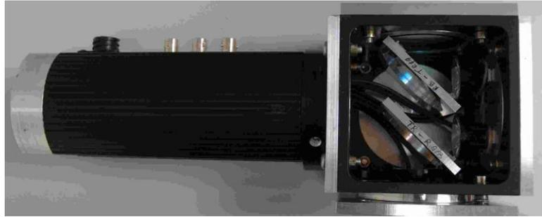
**Figure 5. Tri-color RGB LED Lamp used for High Speed Color PSV Measurements.**
