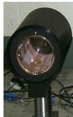
Packaged I2S-5 with integrated thermocouple and heating element in aluminum housing.
