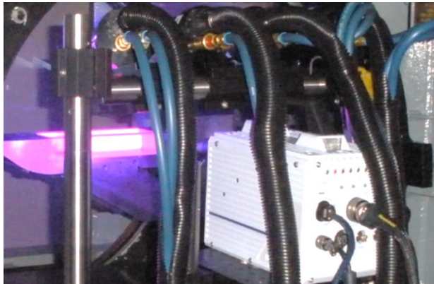
Fast PSP in a Subsonic Cavity Under UV Excitation (Left), Standing Pressure Waves in a Subsonic Cavity (Right), (Courtesy: US Air Force)
