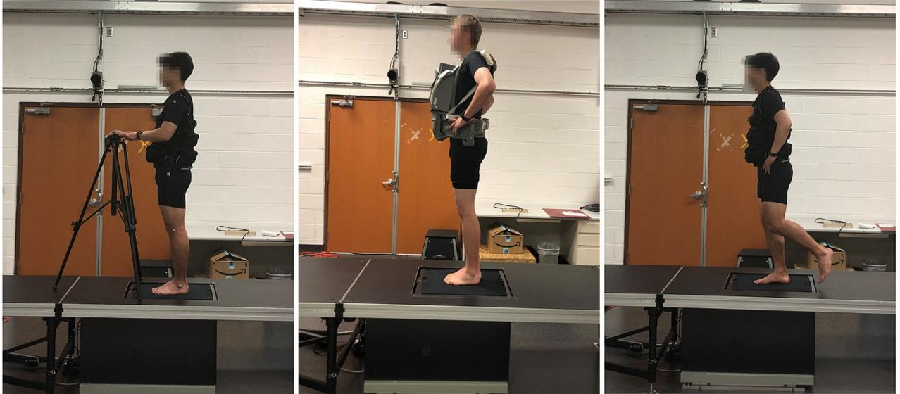
**Fig 1. Raised platform/walkway, weight conditions, and standing tests.** Left: Static trial with evenly distributed (EV) weight. Middle: Bilateral-foot standing trial with front weight (FV). Right: Single-foot standing trial with EV.
