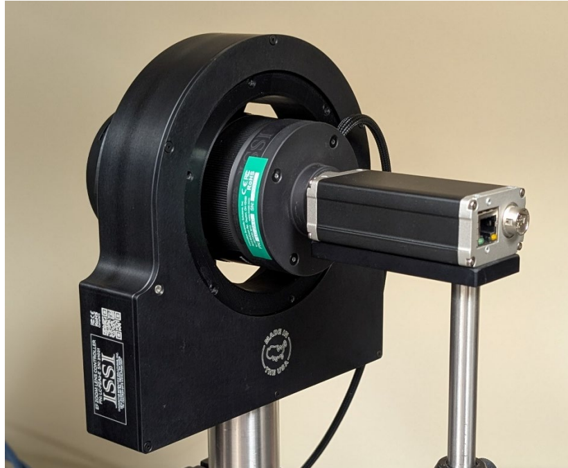
Connection of LC-PZA2-E to EF Lens using LC-2A-C lens adapter on c-mount camera
