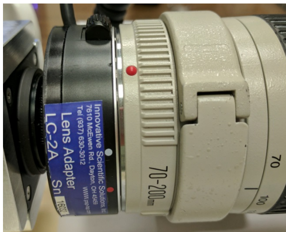
Lens in Lock Position
