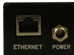
Ethernet / Power Connection
