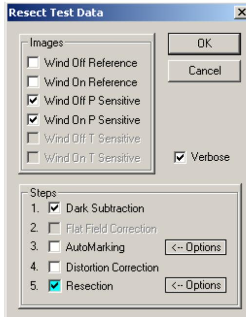
3. In Resection Procedure Dialog (Fig. 7.5) select Wind Off Pressure and Wind On Pressure bitmaps for resection. Don't use for this sample "Automarking" function - all markers are already available. Dark Subtraction is necessary, but Flat-
