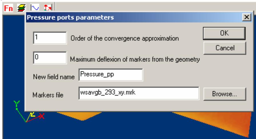
4. In "Pressure Port Parameters" dialog (Fig. 9.2) set order of approximation (maximum is 2) and maximum deviation between pressure port coordinates and corresponding point on the model mesh. This deviation is determined by accuracy of pressure coordinates measurements on the model and accuracy of the model mesh. Browse and select Markers file (sample is located in Step\_9 folder). Select new field name which will be used to store corrected field values.
