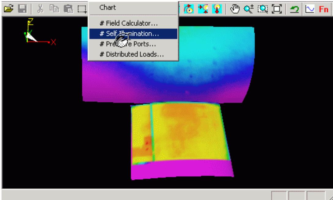
5. Select "Self Illumination" function from "Tools" menu (Fig. 7.8) and set parameters in the Self-Illumination Correction Dialog (Fig. 7.9 and 7.10)
