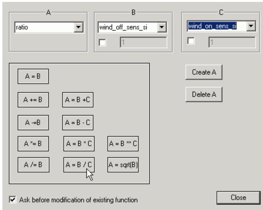
8. The first step here (Fig. 7.13) is creation of the new field "A" (Use "Create A" function), "ratio" was used as the name. Specify B and C components as "wind\_off\_sens\_si" and "wind\_on\_sens\_si" correspondingly, and use "A=B/C" to calculate "ratio" field (Fig. 7.14)
