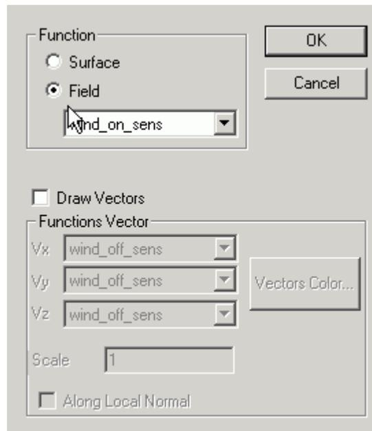
4. Choose appropriate function for presentation in "Fn" dialog (Fig. 7.6). Now you have "wind\_on\_sens" and "wind\_off\_sens" intensities mapped on the 3D mesh - "Field" and mesh itself - "Surface" (Fig. 7.7)
