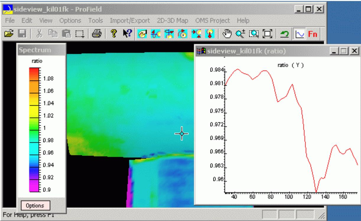
Result presentation. Use "Options" dialog to select dynamic range and LUT. Plot shows (Fig. 7.15, right window) normalized intensity distribution for vertical section where cross cursor is placed.
